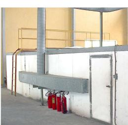
The drying unit is designed to dry the paint coated material. Flash off and drying process is obtained by the forced air circulation which covers the upper and lower surface of the material as it is conveyed along the slat conveyor.
